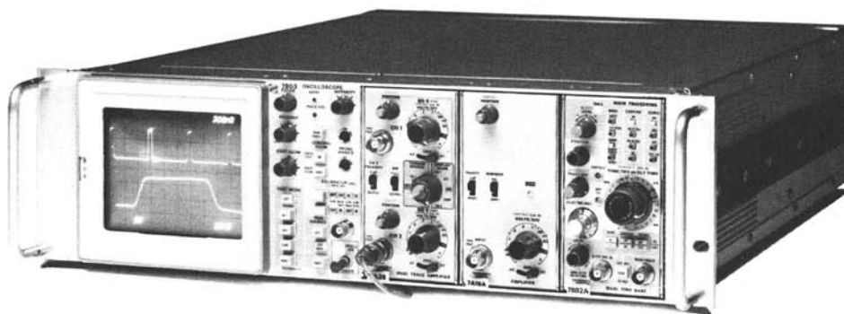
The R7903 requires only 5.25 inches of rack height in a standard 19-inch rack. It is fan-cooled and comes complete with slideout chassis tracks.
